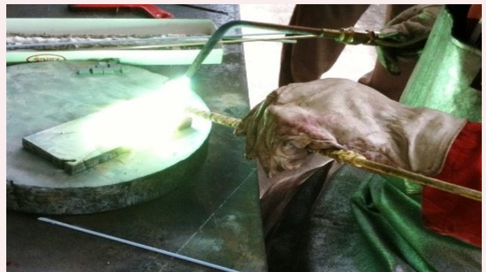
Applying the composite rod with oxy -acetylene torch
